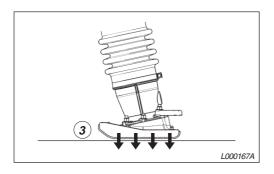
1. Move the throttle to the working mode and the tamper will begin to move.
