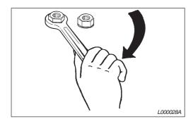
4. Check and, where necessary, tighten screws and nuts.
