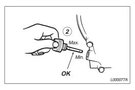
2. Check the oil level in the engine while the tamper is upright.
