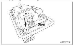
1. Put the throttle in the stop mode. Fuel supply to the engine is cut off in this mode, tank ventilation is closed and the engine switch is Off.
